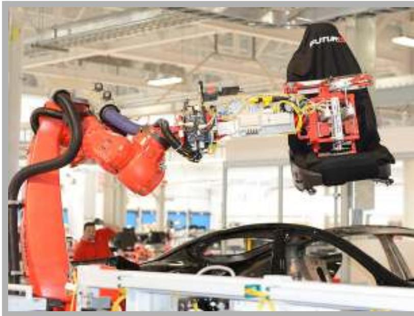
Robots install the Model S seats.
