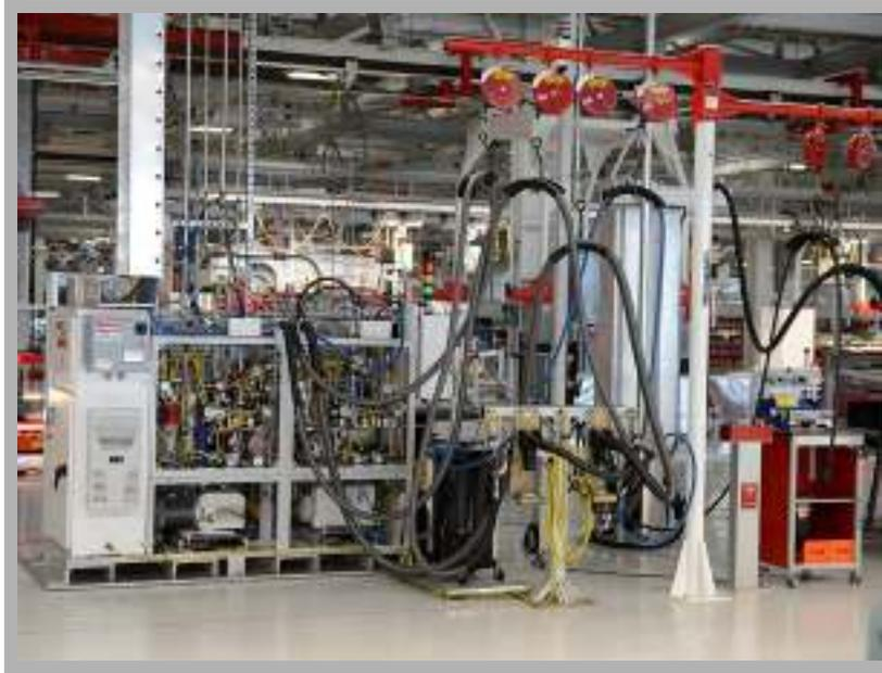
This array of hoses and tubes puts the fluids into the cars near the end of the production line, just before they go through a final quality-control check on an indoor test track.
