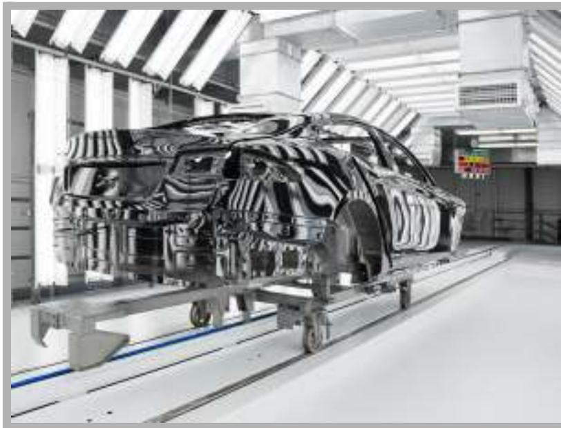
The paint shop uses robots to spray the colored base layer first. This is then covered with a clear top layer for protection and gloss. For premium colors, Tesla uses a three-stage process incorporating a colored base layer, a pearlescent middle layer, and clear top layer. After painting, employees inspect the work in this brightly lit chamber.
