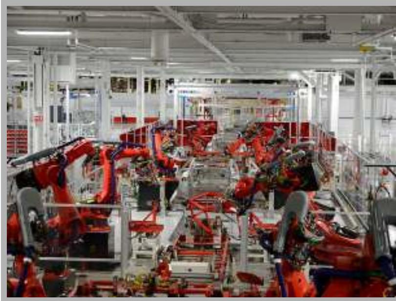
Tesla removed all the old assembly equipment and installed new robots that can perform several different functions, such as assembling the chassis. Some robots are true multitaskers that can weld, rivet, glue, and laser-cut.
