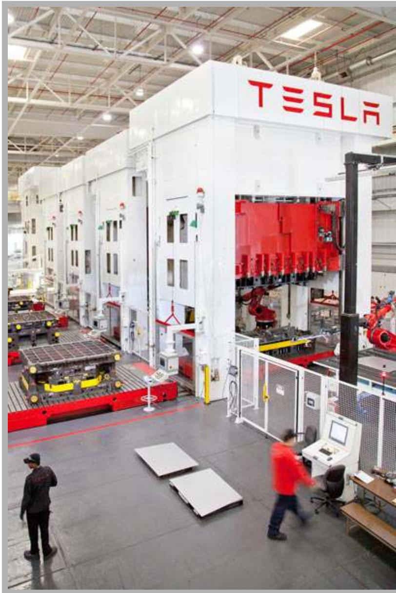
Tesla produces 95 percent of the parts in-house. Huge stamping presses produce aluminum body panels. Resin injection molding machines and die casting create aluminum components. The imported AA-size battery cells—more than 7000 are used in each battery pack—are assembled into the battery packs on the second floor.
