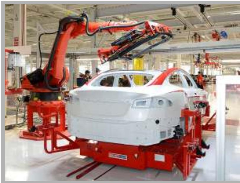
This robot uses high-definition 3D cameras to pick up the sunroof, put glue on it, and then align it correctly on the body.
