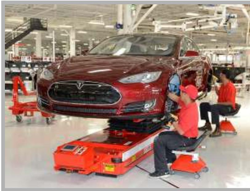
Smart Carts, rather than a fixed assembly line, carry the Model S bodies around the factory during final assembly. The body can be raised or lowered to make it easier for Tesla workers.
