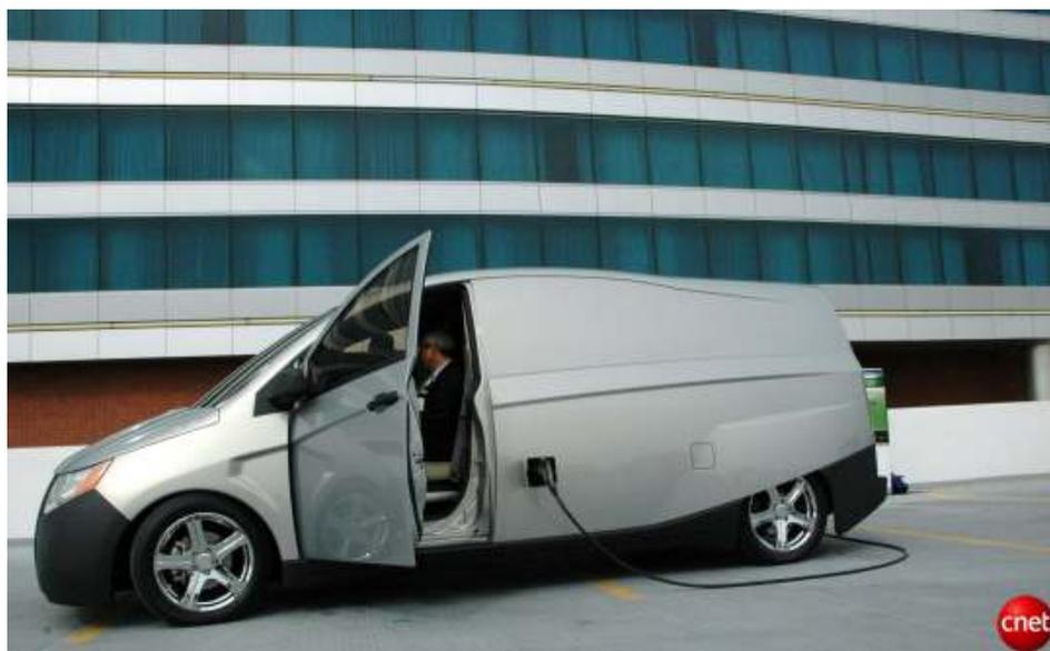
The Idea van used lightweight materials, an aerodynamic design, and plug-in hybrid power to achieve a big jump in fuel efficiency.
