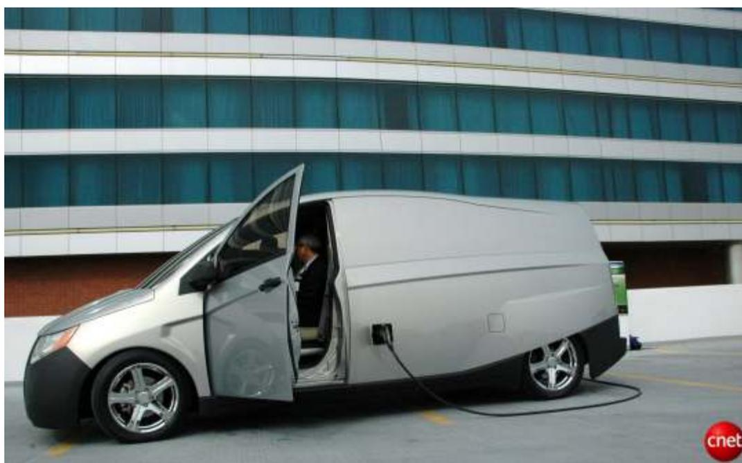
The Idea van used lightweight materials, an aerodynamic design, and plug-in hybrid power to achieve a big jump in fuel efficiency.
