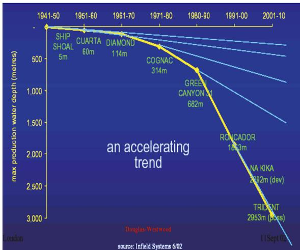
Figure 5 - Deepwater oil and gas developments.
