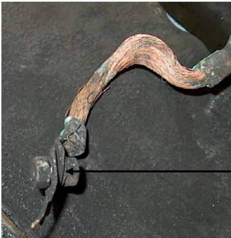
Gap between lug and fuse blade
