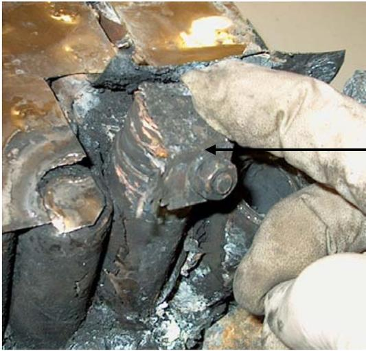
Tab remnant with a portion of the Nickel sheet. This remnant includes the other half of the fuse from Figure 11.
