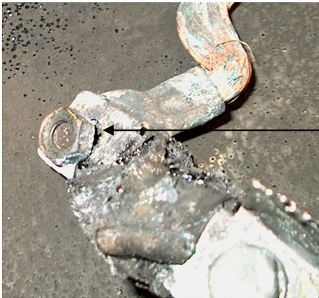
Bolt not protruding through nut. Obvious gap in the bolted joint.
