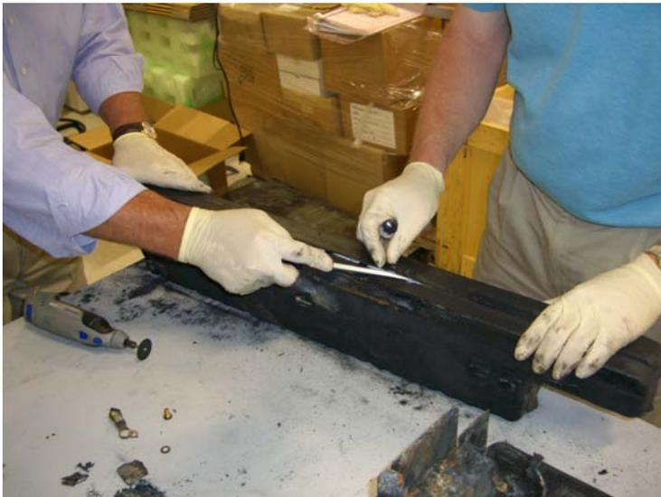
With the batteries removed from the tray, the terminals on the left-hand end (non-fused) could be more closely examined. On all four batteries, these connections were found to be loose (Figure 14).
