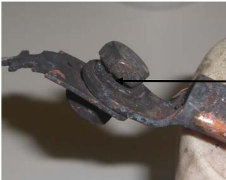
Washer located under bolt head. No spacer between lug and fuse blade
