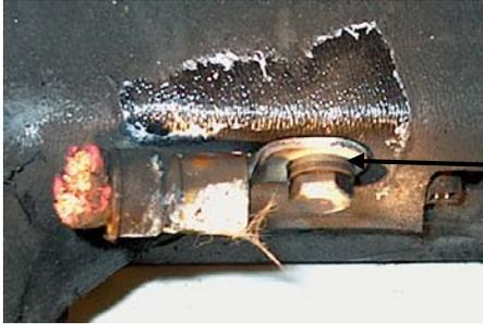
Spacer (washers) placed between bolt head and lug—lug contacting plastic housing
