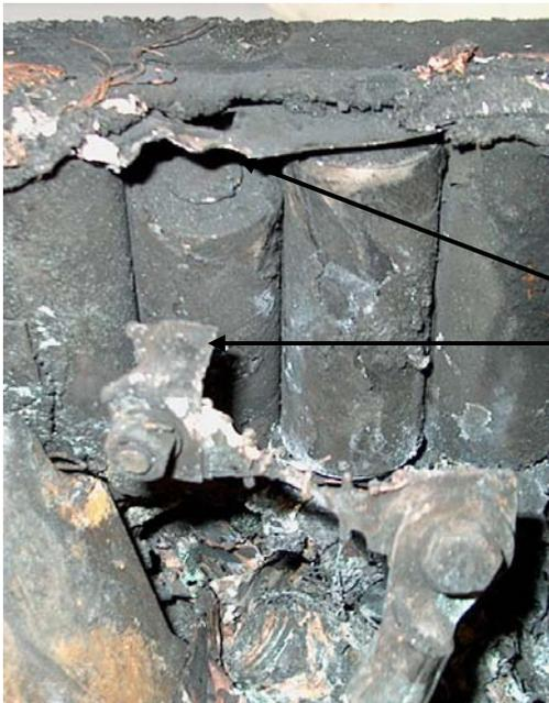
Tab remnant connected to fuse blade. Location on Nickel sheet where tab was originally located.
