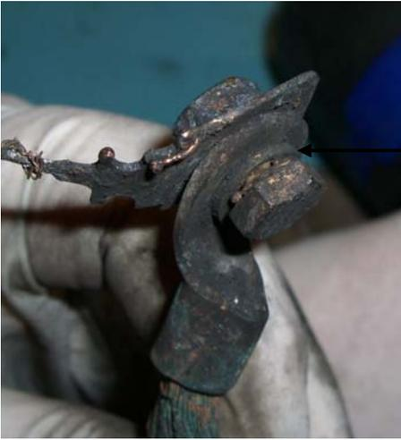
Washer placed under bolt head. No spacer between lug and fuse blade.
