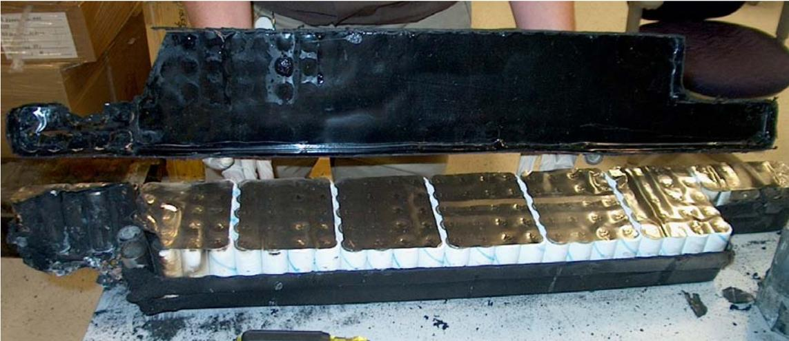
The cells were removed from the clamshell housings to allow for inspection of the cells and Nickel sheets on the bottom side. Nothing unusual (beyond the same burning seen from the top) was noted.
