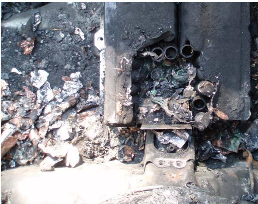
Arcing would have occurred at any area where a short circuit occurred. The ejected material contains electrolyte so it would catch fire in the presence of this arcing. These short circuits along with any burning material caused additional cells to rupture. The inspection showed that all of the ruptured cells were immediately adjacent to this cavity area, indicating that they were exposed to enough heat to cause the rupture.
