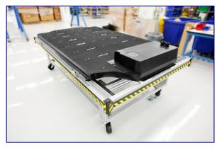
Above: The custom battery pack Tesla uses for its Tesla Model S. Inside are hundreds of lithium cells.
