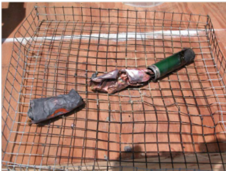
FIGURE 5. EXPLODED CELL AND ITS CONTENTS
