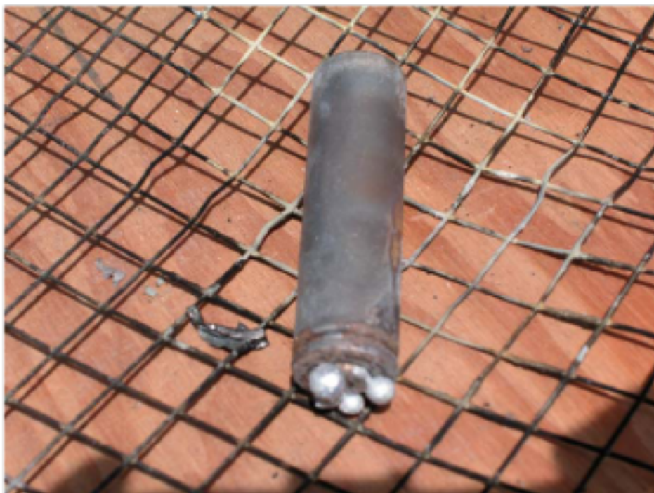
FIGURE 4. EXPENDED CELL WITH METALLIC BEADS ON POSITIVE TERMINAL
