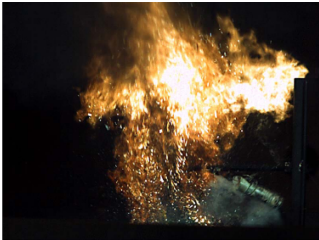
FIGURE 9. HIGH-SPEED VIDEO CAPTURE OF EXPLODING CELL
