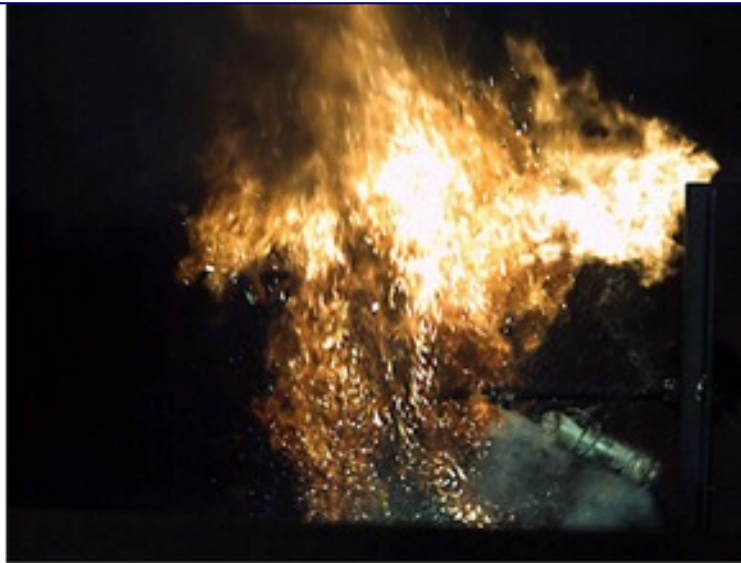
FIGURE 9. HIGH-SPEED VIDEO CAPTURE OF EXPLODING CELL
