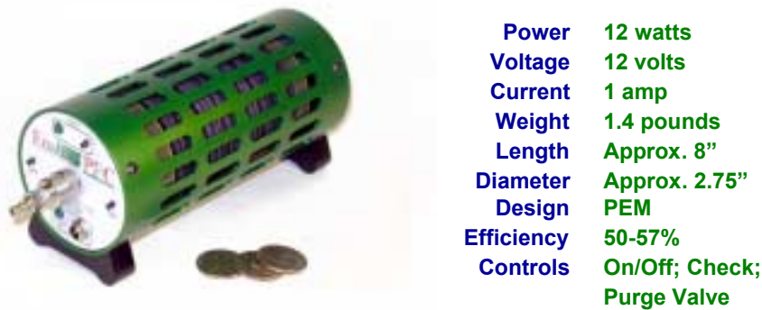
Figure 2 – Photograph and specifications of the Enable™ 12 Watt PFC.
