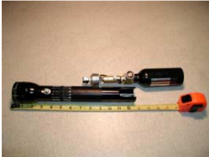
Figure 8 – Flashlight housing, fittings and hydride.
