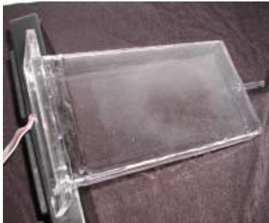
Figure 8: Sensor chamber showing exhaust tube at the right.
