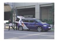
Along the same lines, GM's latest prototype, an advanced version of the HydroGen3 released in December, 2002, is the first fuel cell vehicle to incorporate a 10,000 pounds per square inch (psi) hydrogen storage tank, at least double that of any previous fuel cell vehicle. Additionally, GM's liquid hydrogen fueled HydroGen3 prototype will be its first fuel cell vehicle used by a private company, FedEx Corp. in
