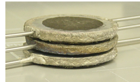
Braze gas tubes Slurry-coat cathode
