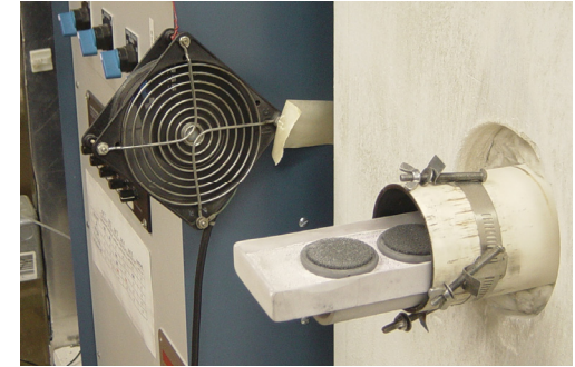
Sinter in single high- temperature process
