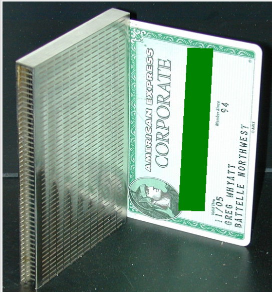
Reforming Reactor Panel
