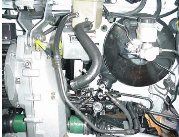
Figure 13 View of engine compartment prior to fuel cell installation showing Solectria 78 kW electric motor, gearbox, and Ford electric power steering, and vacuum brake assembly.
