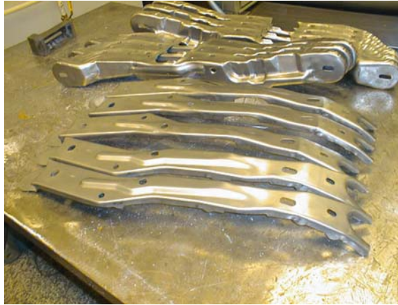
Figure 8 Pre-assembly custom components of alloy sub-frame.
