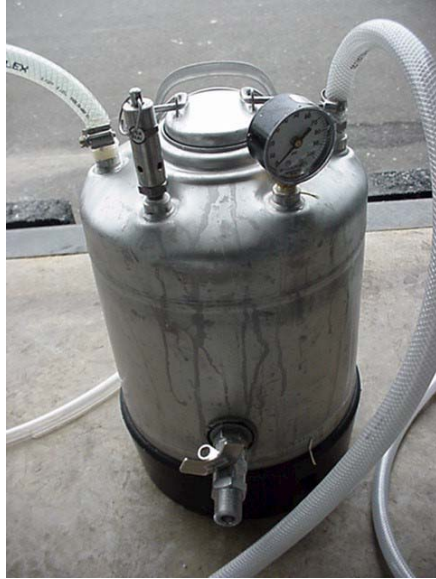
Figure 38 Hydrogen generator test stand condenser water reclamation tank used to develop hydrogen generator design prior to installation in the vehicle.
