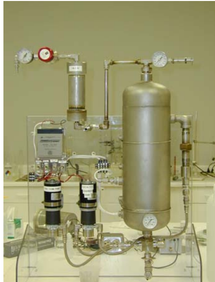
Figure 36 Millennium Cell, Inc. Hydrogen Generator Model 1 designed to power a 1.2 kW fuel cell.
