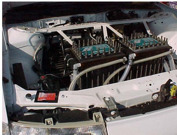
Figure 42 Two 7 kW (gross) fuel cell stacks installed in Genesis vehicle.
