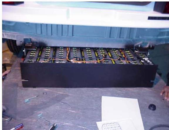
Figure 18 Rear battery pack partially installed in the Genesis.
