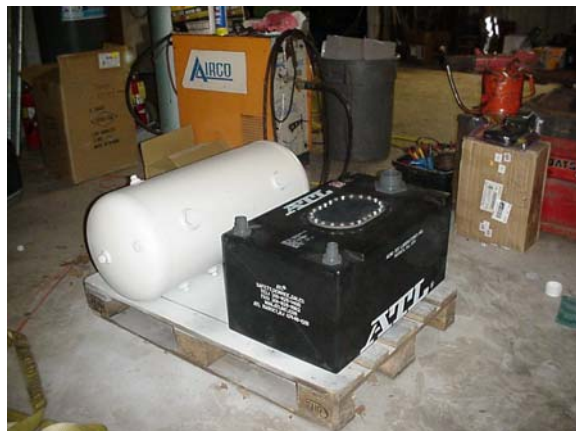
Figure 6 Spent fuel condensate / sodium borate tank (left) and fuel tank (right) prior to installation in genesis vehicle.
