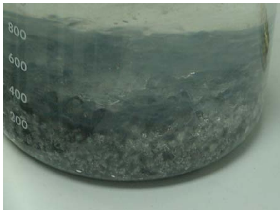
Figure 7 Crystallized sodium borate byproduct of reaction.
