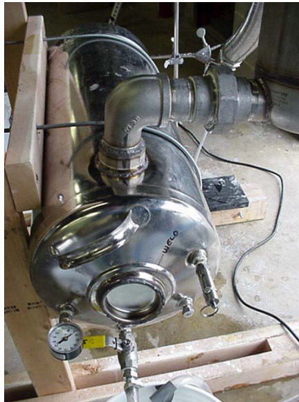
Figure 37 Millennium Cell, Inc. hydrogen generator test stand used to develop hydrogen generator design prior to installation in the vehicle.
