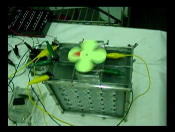
MFC webcam (live video of an MFC running a fan) www.engr.psu.edu/mfccam
