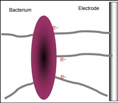
Bacteria that can transfer electrons directly to the electrode:
