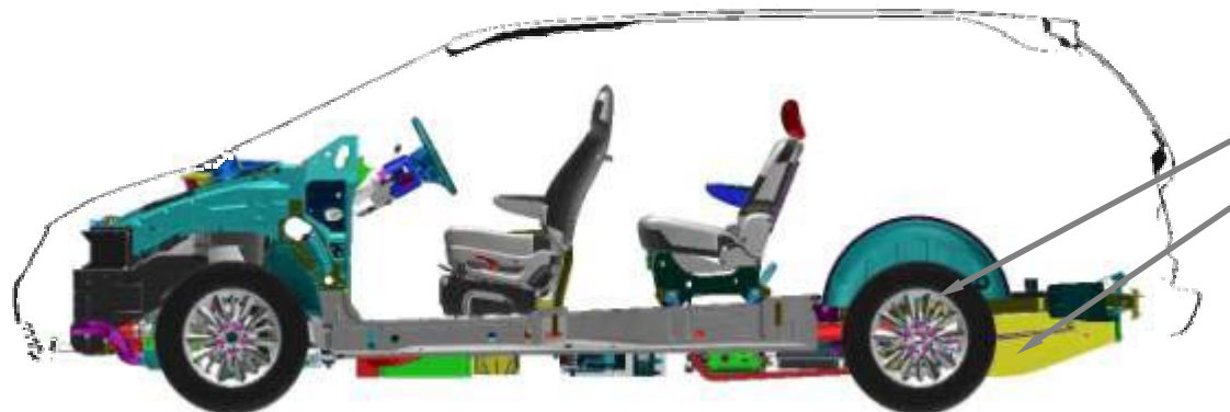
Hydrogen On Demand™ H 2 generation system, fuel and borate tanks (Equals energy storage of about 5 compressed tanks)
