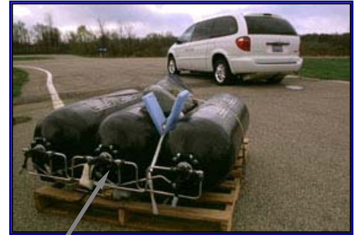
Compressed H 2 cylinders (3 tanks @ 5,000 psi)
