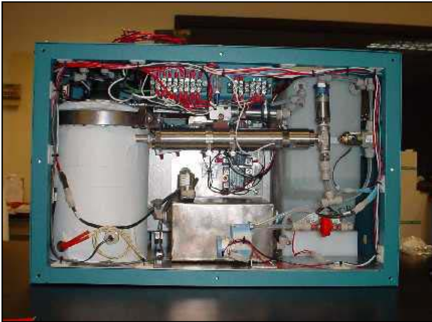
Hydrogen on Demand™ (3 hour runtime @ max load) 1.2 kW hydrogen generation system
