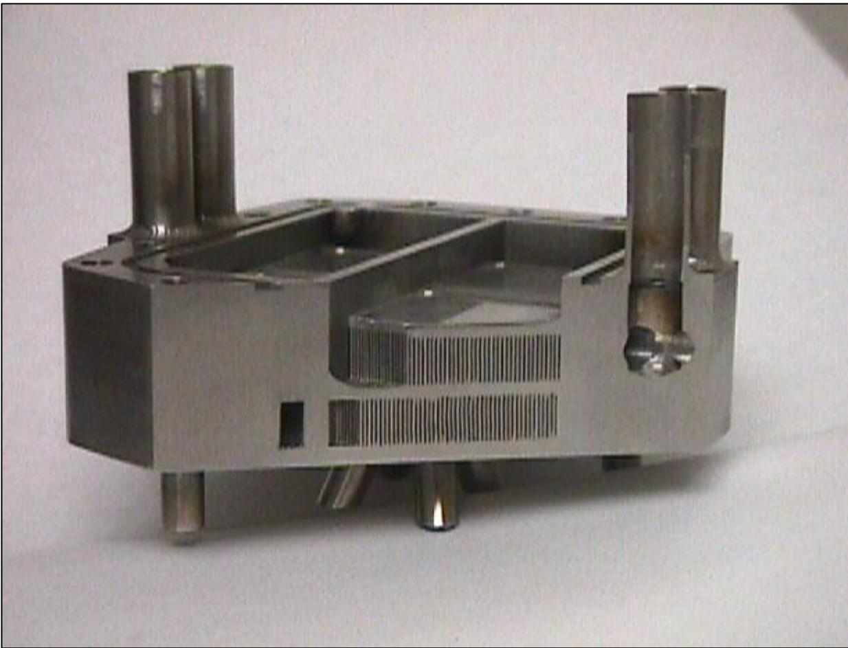
Battelle 50 kW microchannel integrated combustor-gasoline vaporizer. Full size unit, ~ 13 cm at longest dimension.
