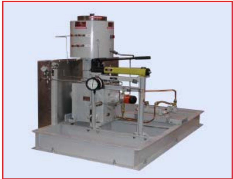
Hydrogen Compressor, Discharge Pressure = 6000 psig (400 bar), Capacity = 30 scfm (48 Nm 3 /hr)
