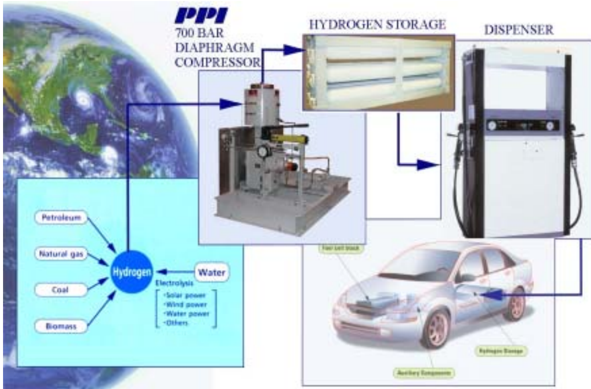
Hydrogen Compressor, Discharge Pressure = 5000 psig (345 bar), Capacity = 20 scfm (32 Nm 3 /hr)
