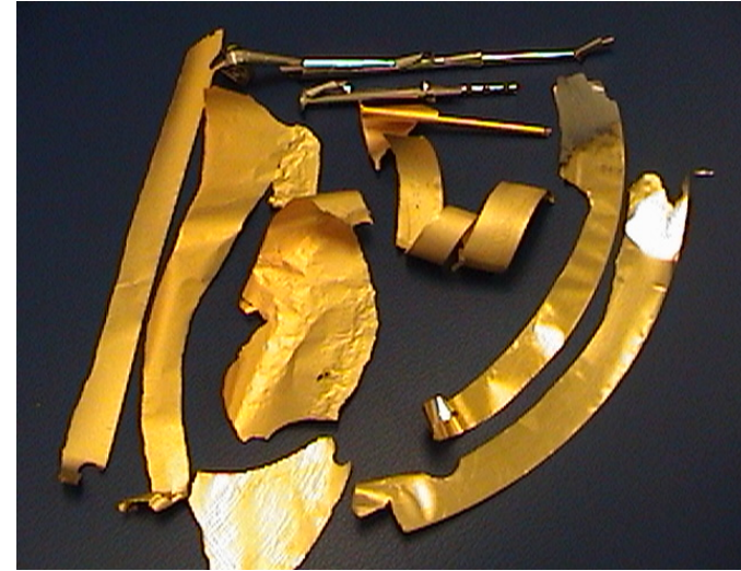
Delaminated metal foils deposited on Stainless steel substrates
