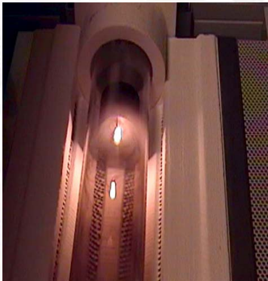
Laser plume during nanohorn production inside tube furnace
