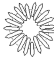
Schematic diagram of nanohorn aggregates. [Bekyarova'02]
