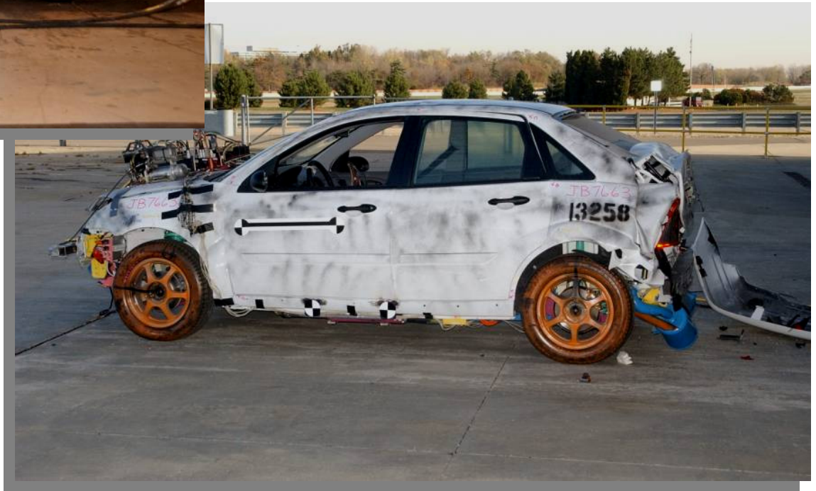
90° 30 MPH Rear Moving Barrier Impact
