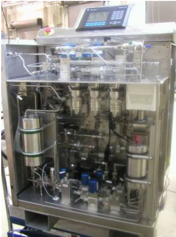
1kW capable URFC test system delivered to NASA
