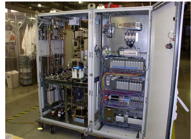
1 kW closed loop DRFC demonstrator ready for test
