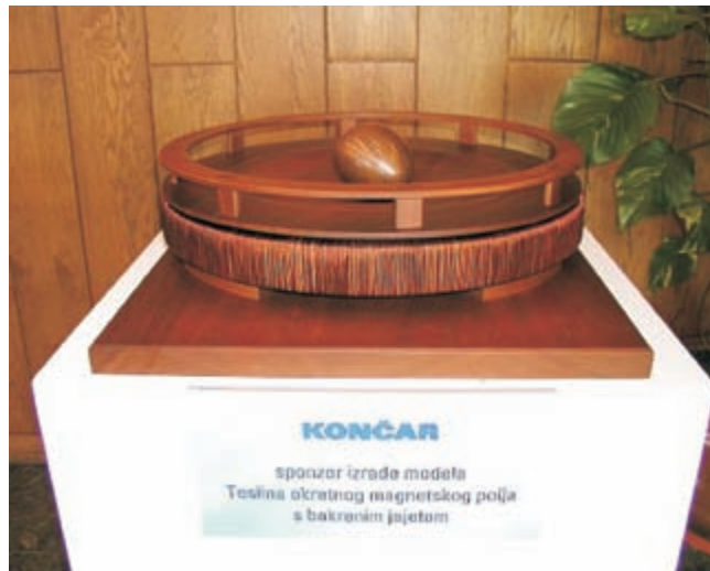
Fig 3 – Demonstration of the effects of rotating magnetic field performed by Nikola Tesla for the first time at the World's Colombian Exhibition in Chicago in 1893
