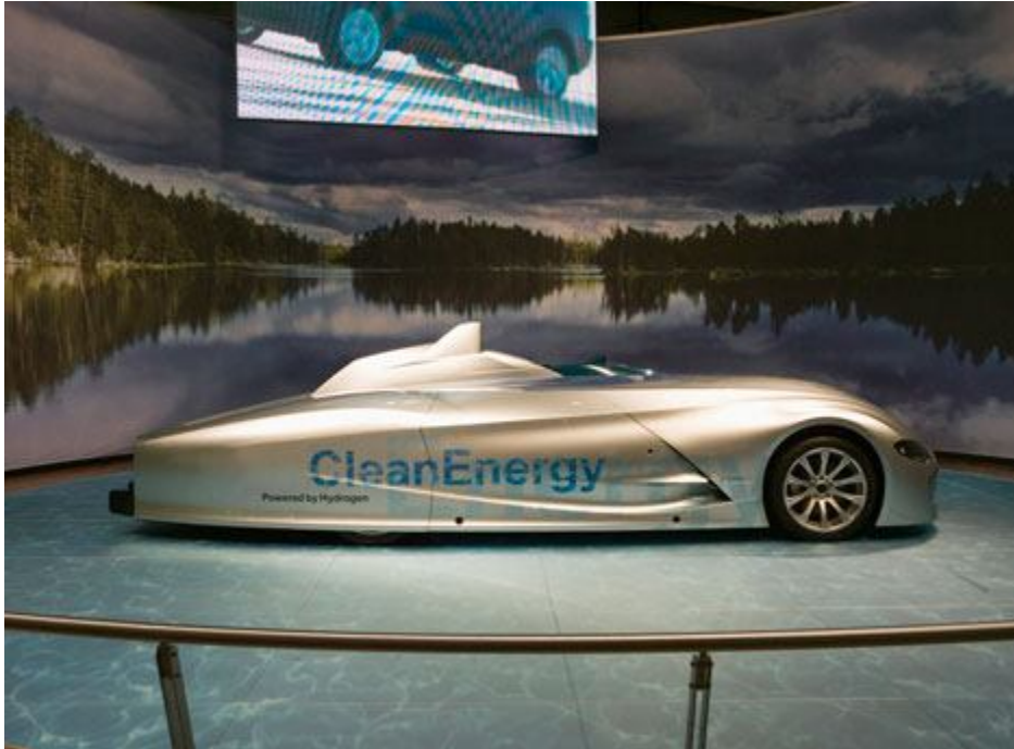
BMW's H2R (Hydrogen Record Car) is powered entirely by the clean-burning process of liquid hydrogen combustion. This futuristic race car has already set nine speed records of 300 km per hour and above.
