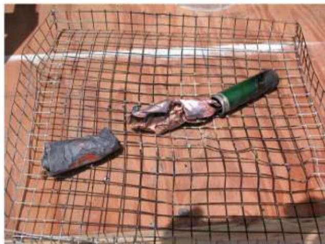
FIGURE 5. EXPLODED CELL AND ITS CONTENTS
