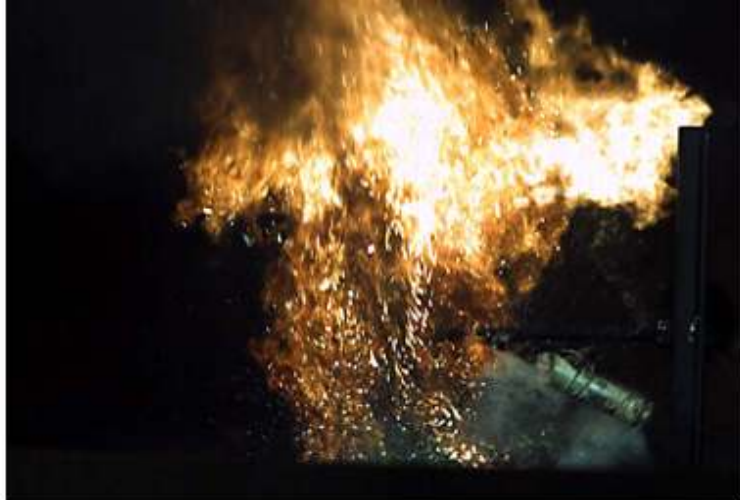
FIGURE 9. HIGH-SPEED VIDEO CAPTURE OF EXPLODING CELL
