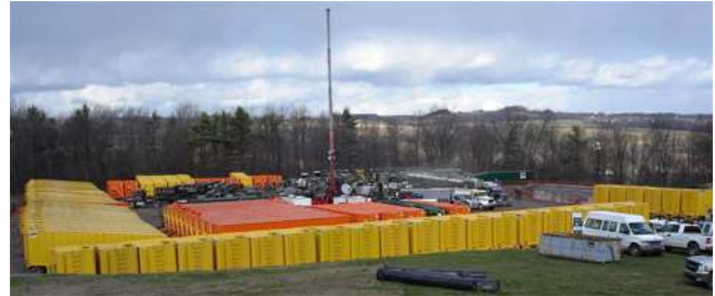
A hydraulic fracturing operation in Bradford County, Pa. It's possible that for each modern gas well drilled in the Marcellus and places like it, more than three million gallons of chemically tainted wastewater could be left in the ground forever. (Photo courtesy of the New York State Environmental Impact Statement)
