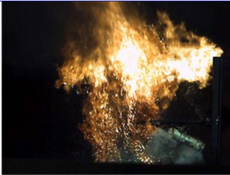
FIGURE 9. HIGH-SPEED VIDEO CAPTURE OF EXPLODING CELL
